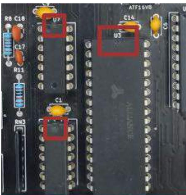
For the DIP components, there is a small *\*u\** at the top that shall match the *\*u\** marking present on both the socket and the PCB silkscreen, as shown on the picture on the left:
