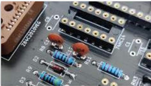
They must be soldered in footprints marked **C17** and **C18**. They can be put in not particular direction.
