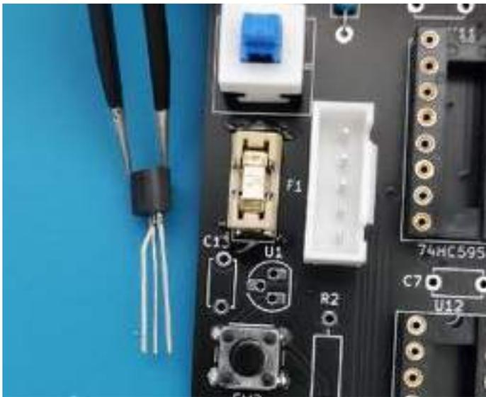
The middle pin must be bent to the back (the front being the flat surface), just like the picture above
