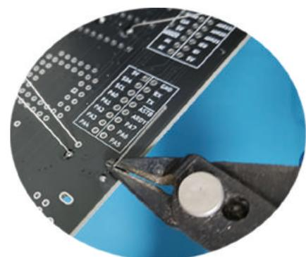
"After soldering the resistors, put on safety glasses, use wire cutters to trim their legs. Cut the legs close to the soldering point without leaving any extra bits that could scratch your hand when touching the board's underside.
