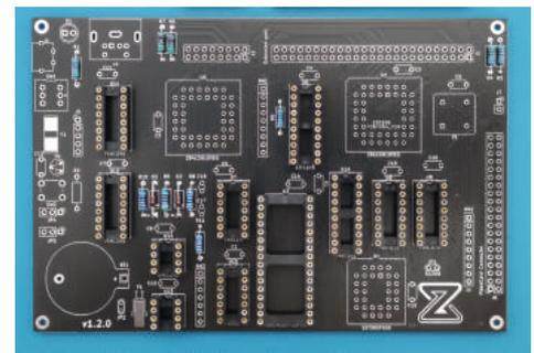
Tip: Using kapton tape, blu-tak or a hard surface can help you keeping the sockets in place before flipping the board. If you don't manage to get all the sockets in place when flipping the board, it is okay, solder them one by one!
