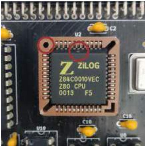
1. Make sure the components are put in the right direction. For the PLCC components, the squared ones, there is a dot on the top, that shall be placed as close as possible to the socket's dot, located on the top left corner. The following picture takes the Z80 CPU as an example:
