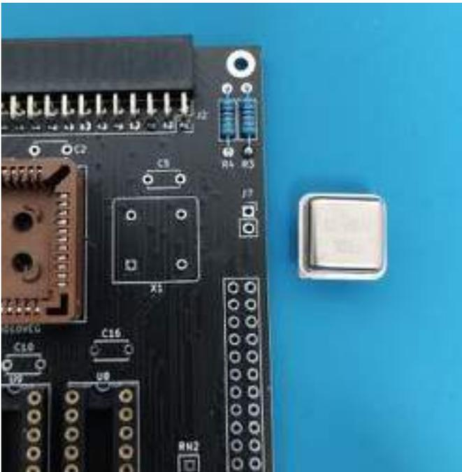
The squared side of it should be located at the bottom left, just like shown on the PCB. It should look like this:
