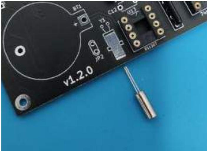
The footprint, referenced **Y1**, shows how it should be soldered. There is no direction this time for this component.
