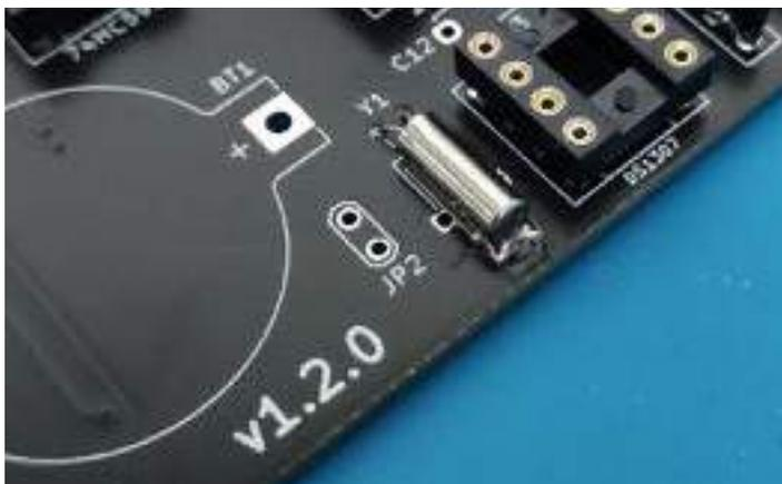
After soldering the two legs, apply some solder between the oscillator case and the footprint on the top of the PCB. It will guarantee that the case is connected to *GND*.
