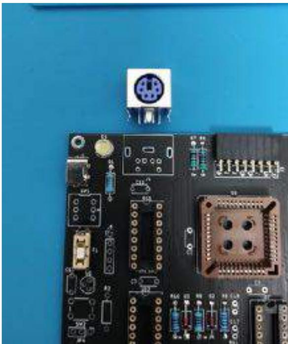
The PS/2 connector, referenced **J4**, must be soldered just by the LED.
