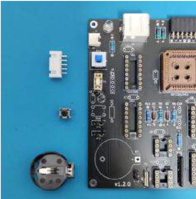
The internal I2C connector, a standard XH 2.54mm connector, should be soldered with the lock on the right.
