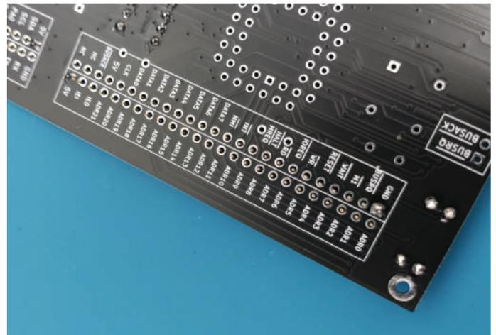
solder the diagonal pins to stabilize the boards
